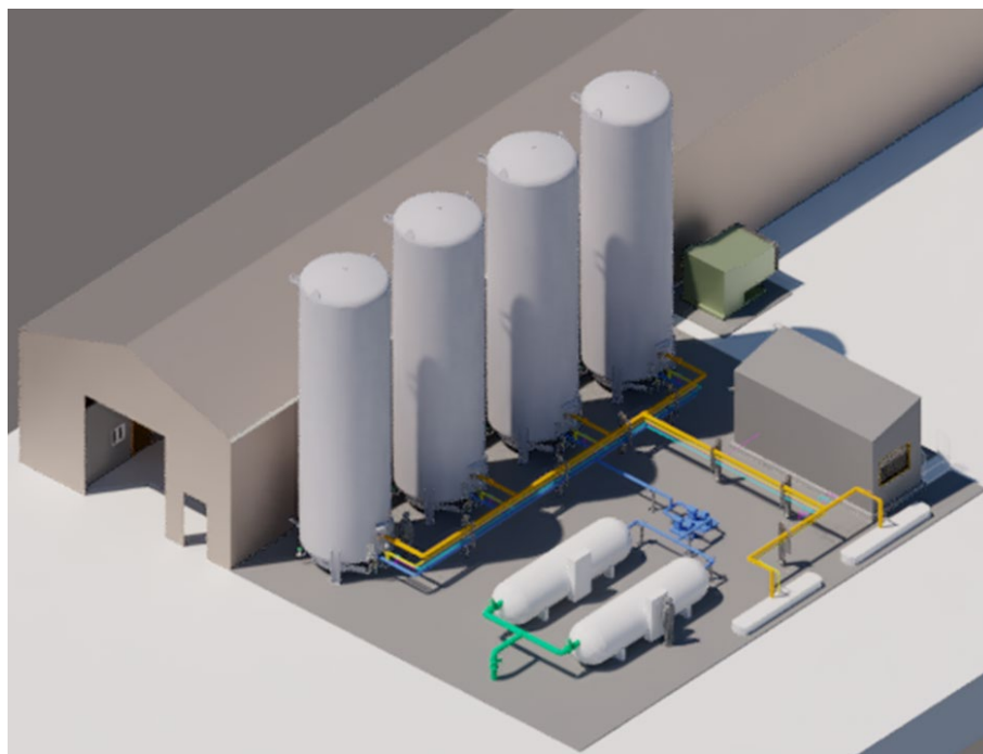
Figure 4. Conceptual design of the Argon Receiving Facility.
